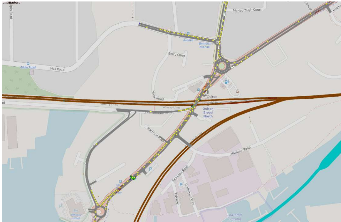
Figure 3.413641: – Base PM congestion at Mutford Peak Normanston Drive/Bridge (5min Bascule Bridge Road (10 min lift – 08:41 after reopening to vehicular traffic)
