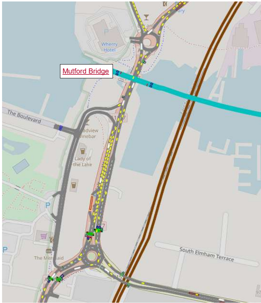
Figure 3.35 – Base AM Peak Mutford Bridge (10 min lift – 08:41 after reopening to vehicular traffic)
